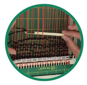
Tie a notch to the weaving shuttle and use the shuttle to take the yarn from one side to the other.
