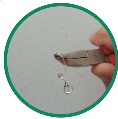
Roll up the legs of the led with small pliers.
